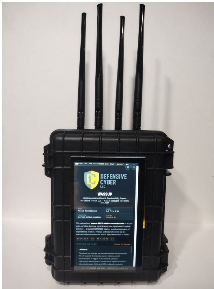
Photo 1 — The WASSUP unit powered on. On boot it comes straight up to the splash screen with the Acceptable Use Policy, ready for the assessor to fill in and acknowledge before the live dashboard opens (see Section 2).
