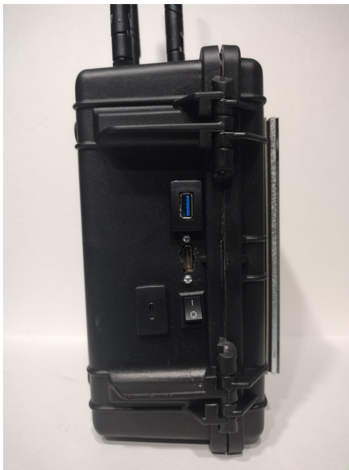
Photo 3 — The left side of the unit. On the right, from top to bottom: the USB-A port, the HDMI port, and the power switch. The USB-C charging port is at the lower middle.
