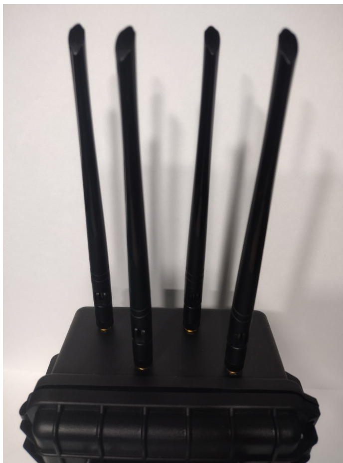
Photo 2 — The top of the unit, where the four antennas mount. They feed the two onboard WiFi adapters, which run in monitor mode so WASSUP can passively capture across the 2.4, 5, and 6 GHz bands at the same time.
